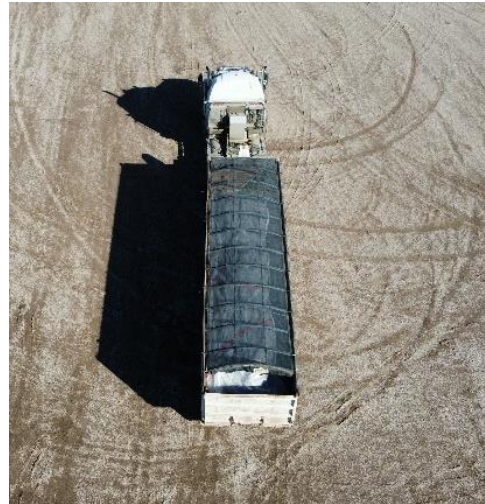
Trailer covered to enclose material during transport
