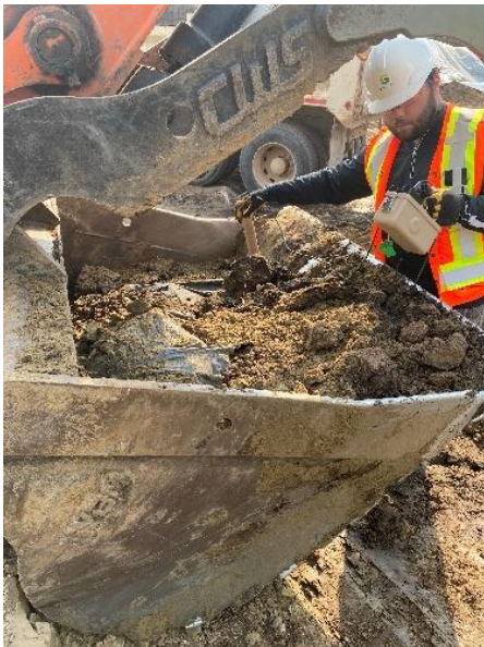
Technician scans excavated material
