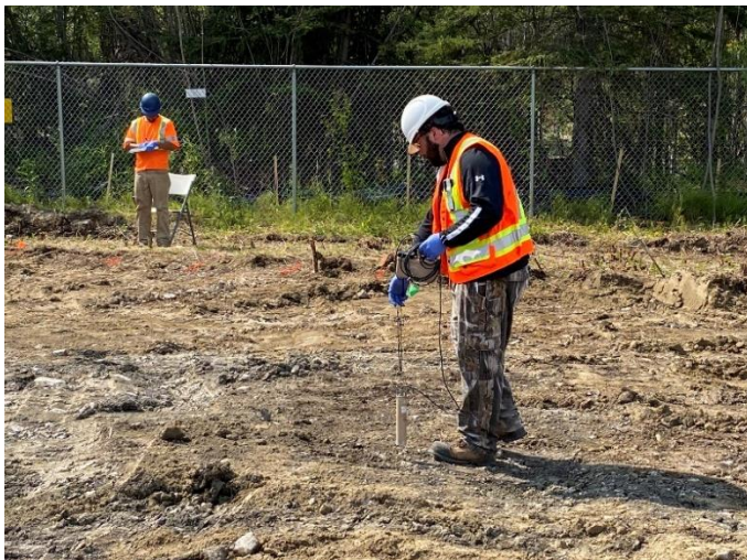
Verification gamma scanning
